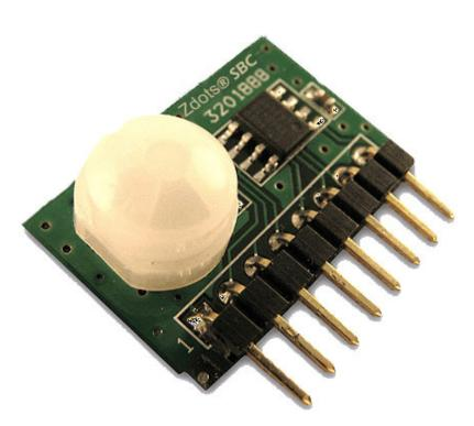
The unique features of the Z8 Encore! XP<sup>®</sup> MCU have permitted a revised look at the traditional PIR based motion detector design. Combined with innovative software techniques, this new approach has overcome the typical performance limitations of the traditional design.
