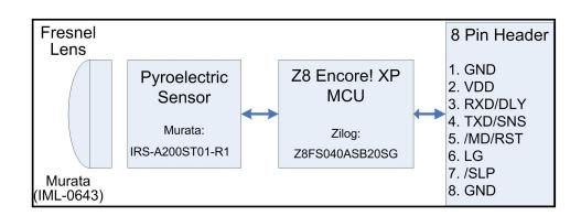
The ePIR Motion Detection Zdots SBC uses a Fresnel lens to break up the radiated IR energy into multiple concentrated images. These images are refracted on to the element of the PIR sensor which generates a signal based on the change in energy. The signal is fed directly to the Z8 Encore! XP MCU where it is analyzed by the motion detection algorithms to determine if it is from a valid source.
